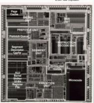
Arithmetic Logic Unit (ALU) (control signals, inputs, outputs), Floating Point Unit (FPU), Prefetching Unit, Registers, ...
