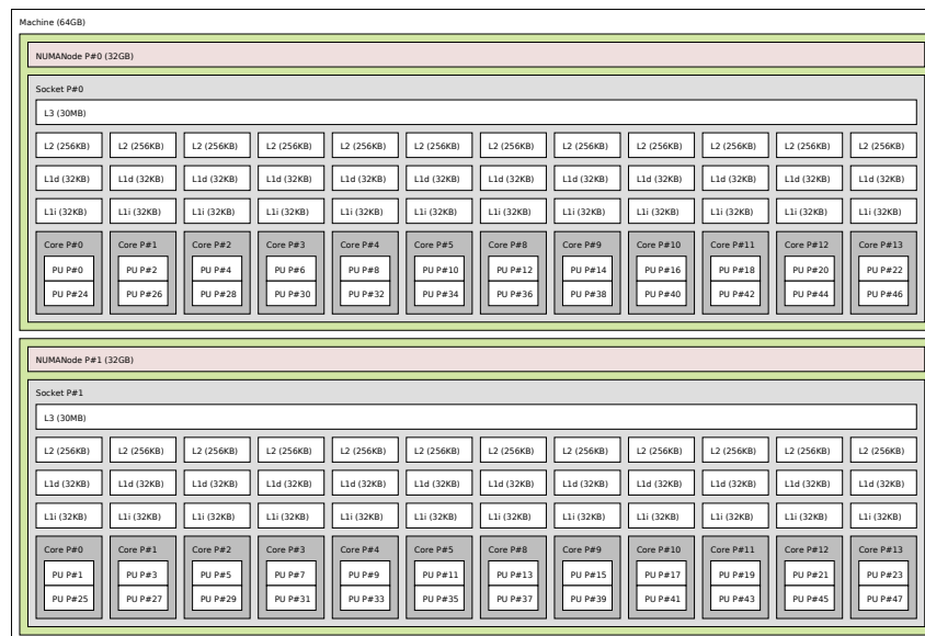
Figure 8: A graphical representation of the hardware specifications of the AICES Haswell nodes.
