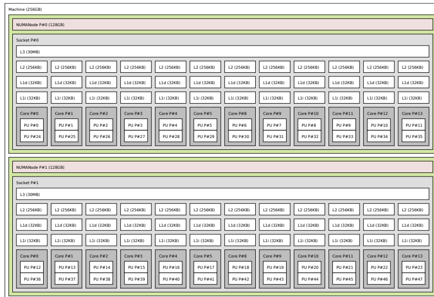
Figure 9: A graphical representation of the hardware specifications of the JURECA nodes.
